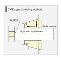
With the material stop mechanism in place, the workpiece does not shift backward during clamping, although there may be slight scuff marks on the surface.
