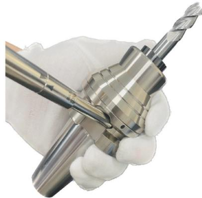
3. Insert a torque wrench into the slot on the side of the toolholder, rotate the wrench clockwise until the two arrows on the wrench surface align. (Please use the original torque wrench from the manufacturer to avoid unstable torque that may cause other issues. Check the hexagonal surface of the wrench for any damage before use.)
