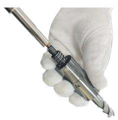
2. Use your hand to insert the collet into the toolholder and rotate it clockwise until the collet is connected to the body. To achieve the best accuracy and clamping force, please clean the inner and outer taper of the toolholder and collet each time you change the tool.
